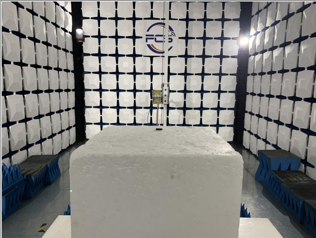
Above 1GHz for radiated emission test setup
