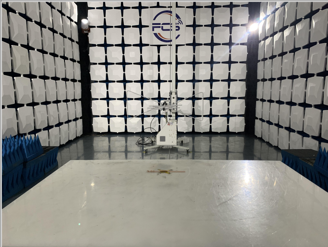
Above 1GHz for radiated emission test setup
