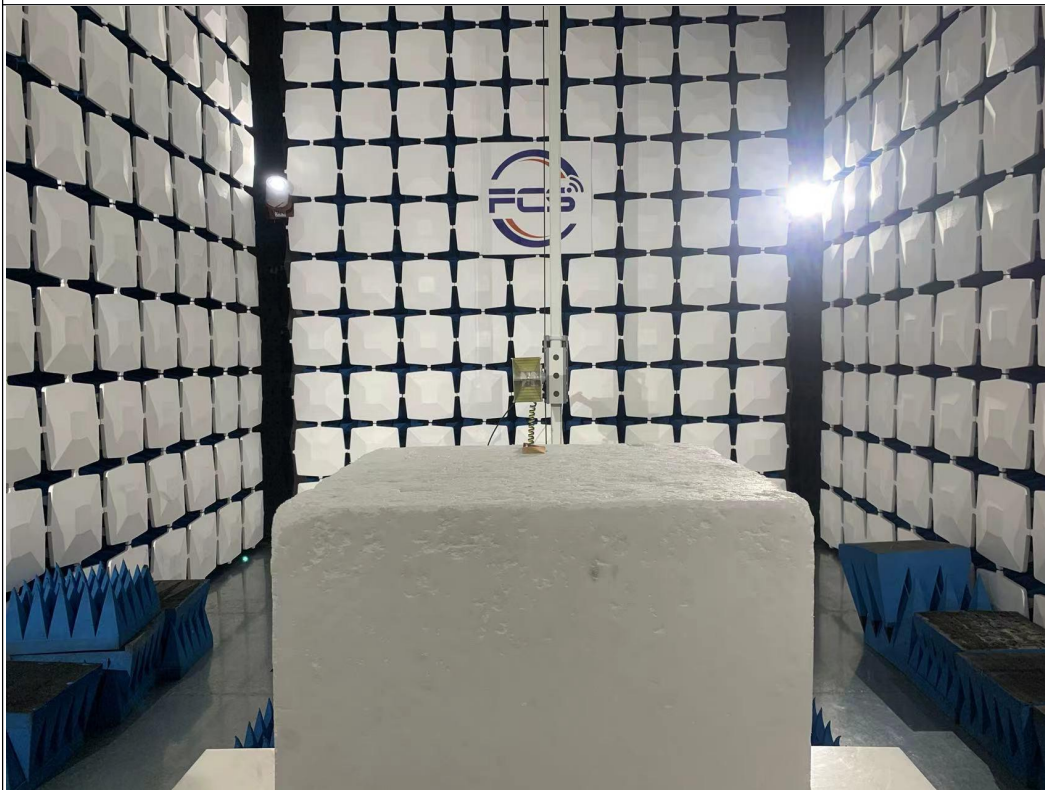
Above 1GHz for radiated emission test setup
