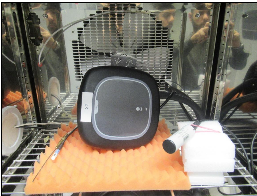
Photo 6 Bench test set up for (99% / 20 dB Bandwidth and Frequency Stability) (@ Ambient + Extreme Temperature, as required)
