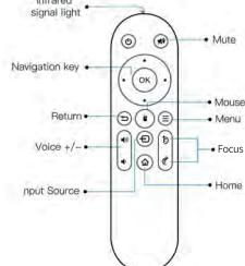
► Remote control shall be working within 5m distance from projector.
