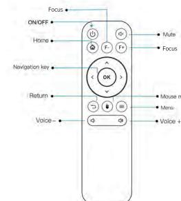
Normal version with infrared remote control
