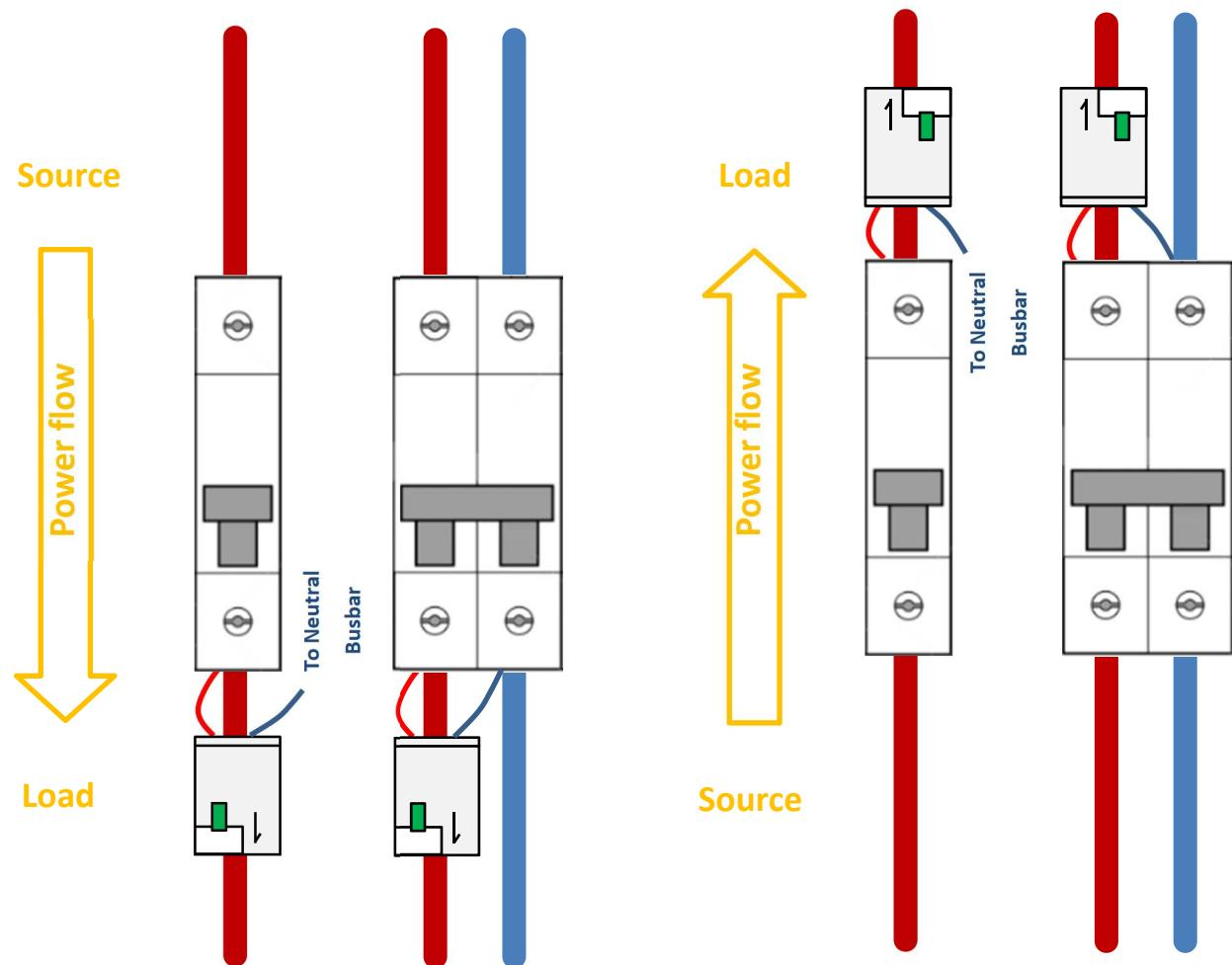
Note: SPM01 can be damaged, if it is installed downstream of switching devices – such as a contactor, frequency converter or motor starters.
