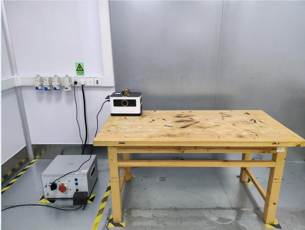
Conducted Emission at AC power line
