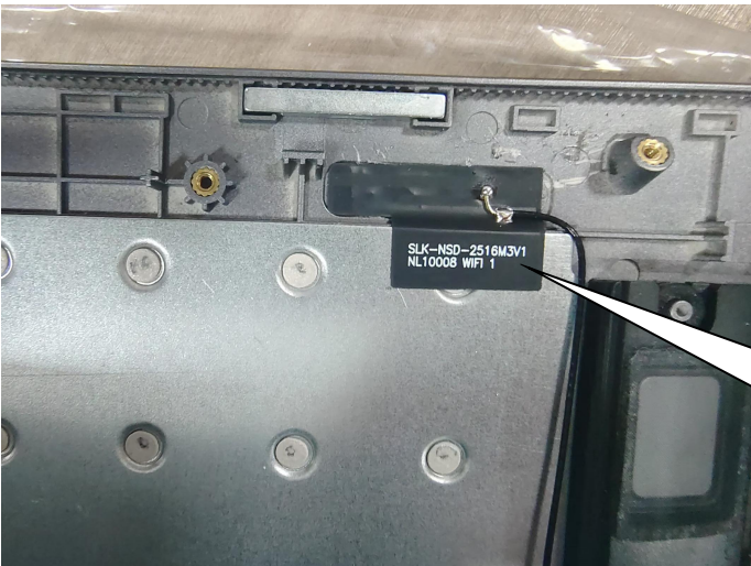
WIFI Main antenna
