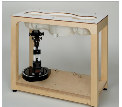
Fig. 8.7 Photo of SAM Twin Phantom
