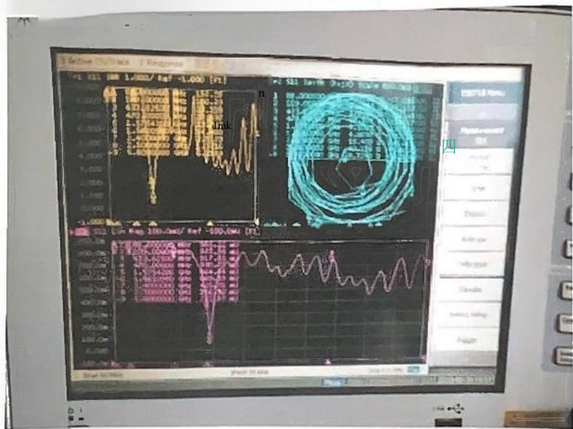
图2 BT 驻波比/SMITH图 Figure 2 BT standing wave ratio /SMITH diagram
