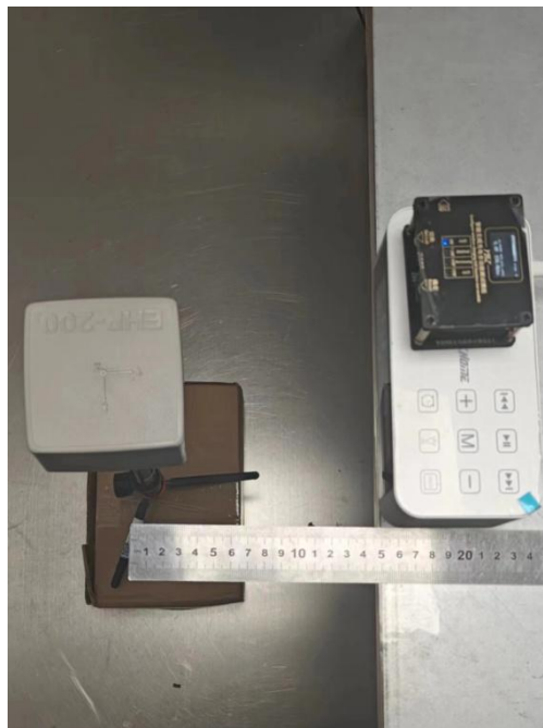
H-Field Strength & E-Field Strength test setup
