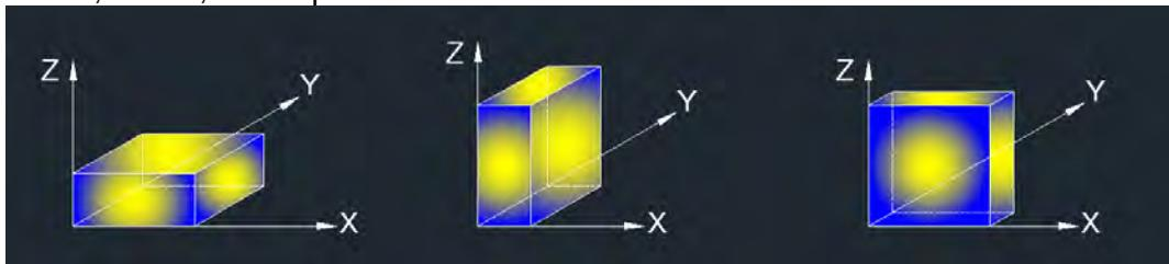
Note 1: For all radiated test, EUT in each of three orthogonal axis emissions had been tested, but only the worse case (Y axis) data recorded in the report.
