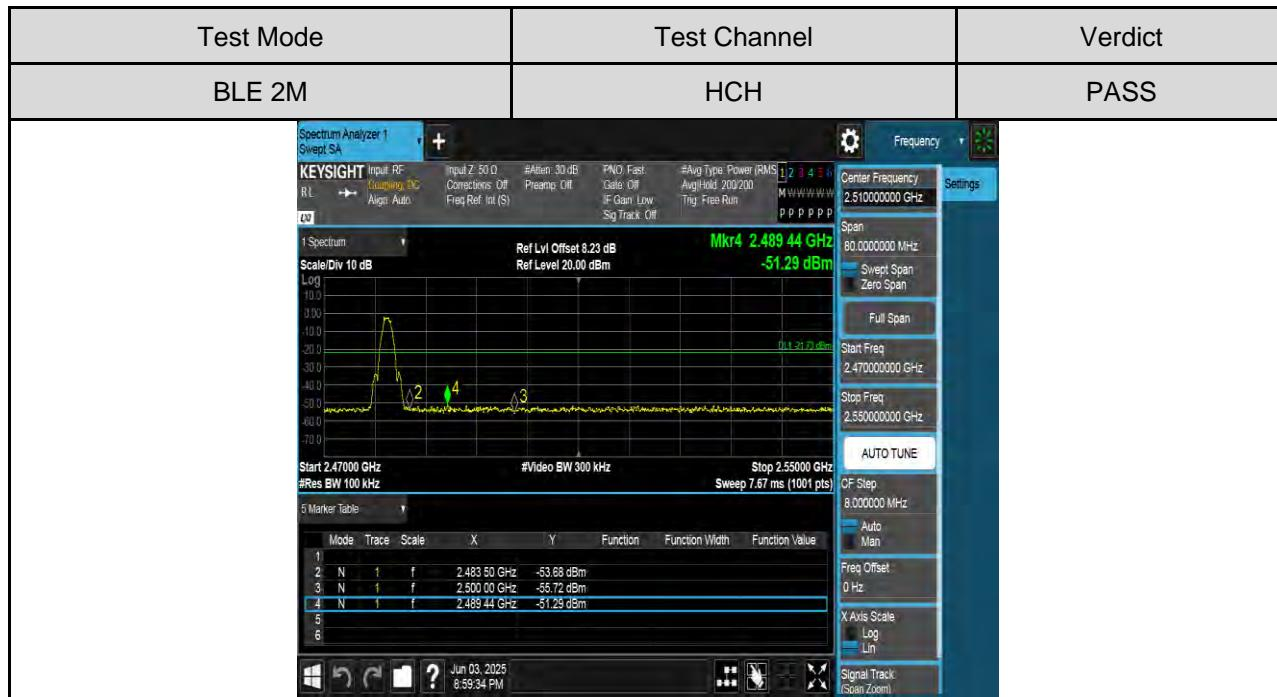
**PART 3: CONDUCTED SPURIOUS EMISSION****TEST RESULTS TABLE**
