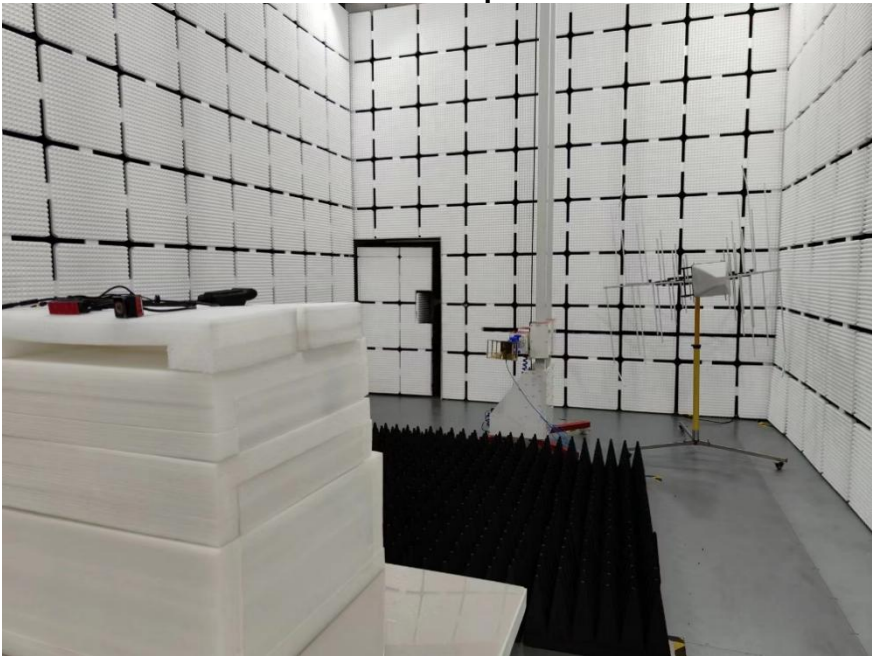
Radiated Emission Test Setup Photo - Above 1GHz
