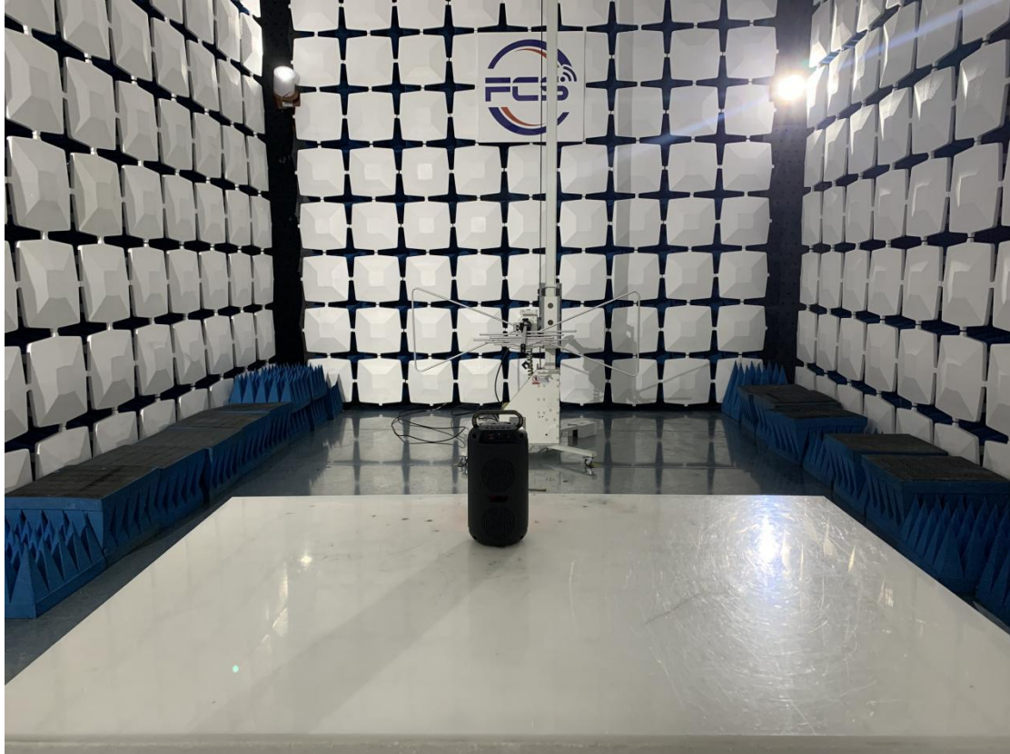
Blow 1GHz for radiated emission test setup
