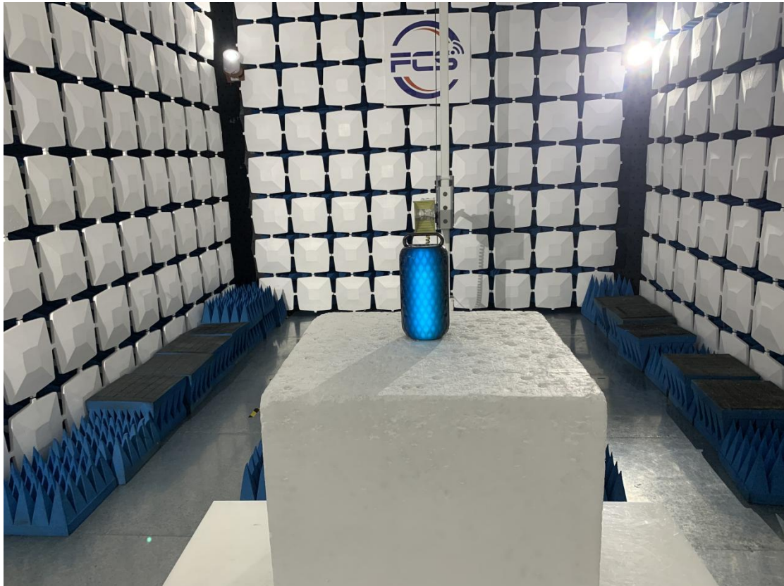
Above 1GHz for radiated emission test setup
