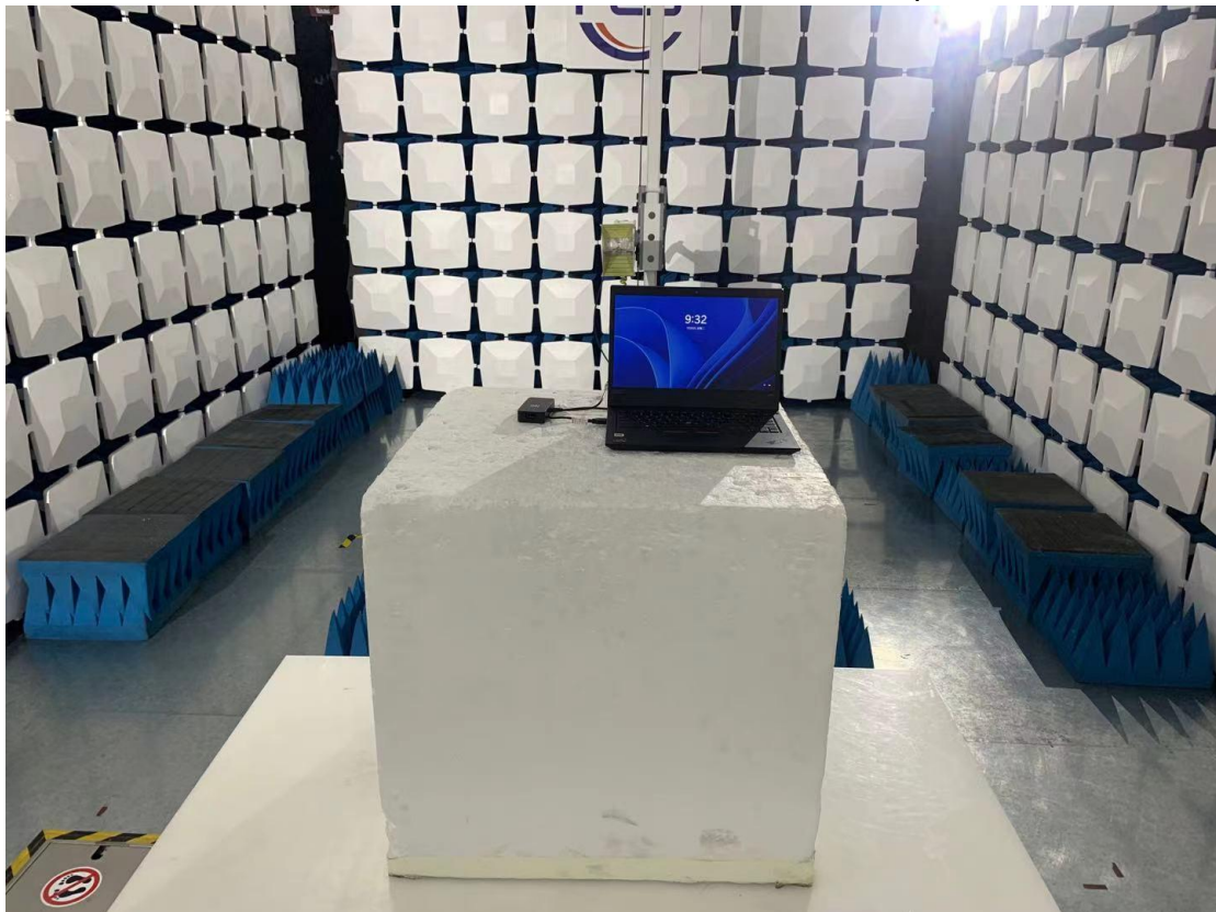
Above 1GHz for radiated emission test setup
