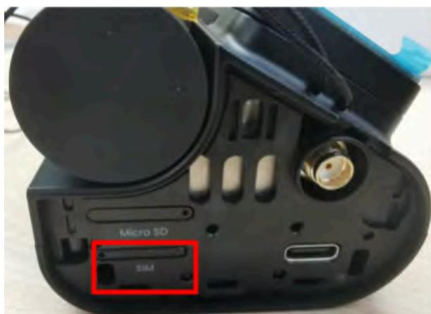
Use needle to pull out the SIM card holder
