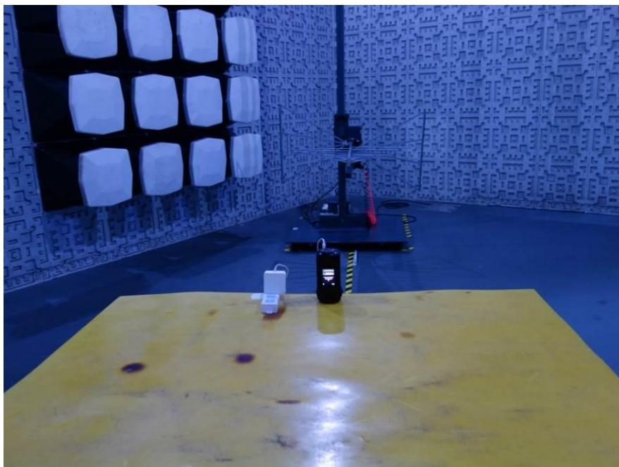
Radiated Spurious Emissions Above 1GHz - Centre of the turntable
