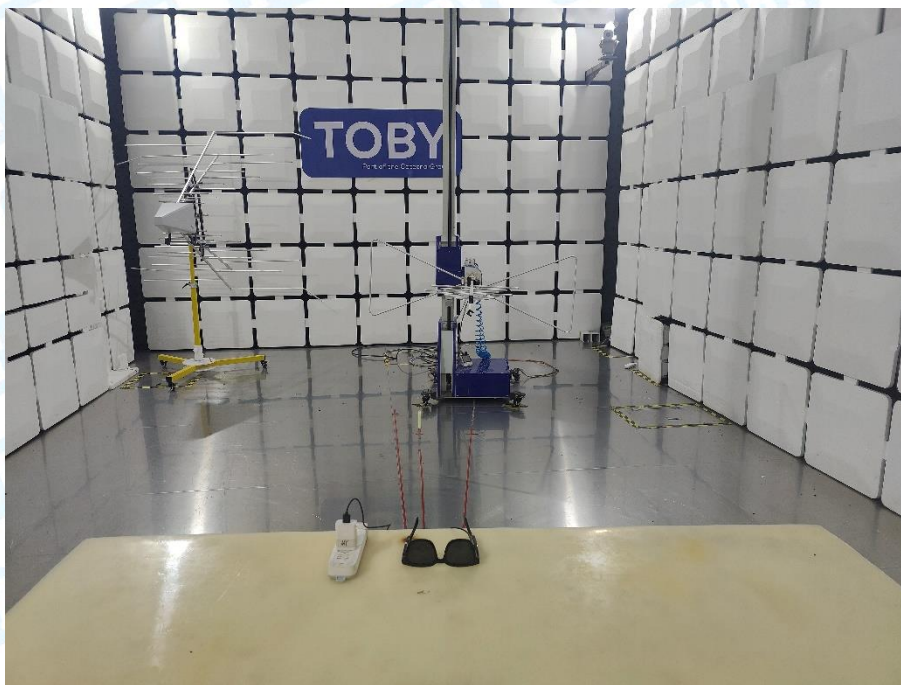
Photo of Setup for Radiated Emission (30MHz~1GHz)
