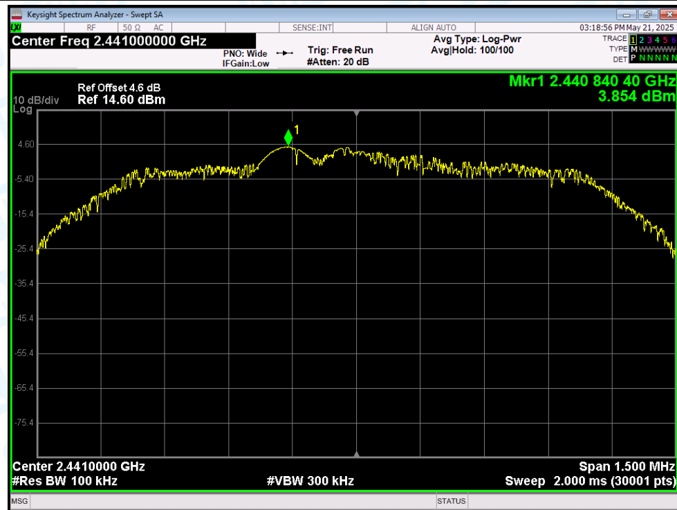
Tx. Spurious NVNT 2-DH1 2441MHz Ant1 Emission
