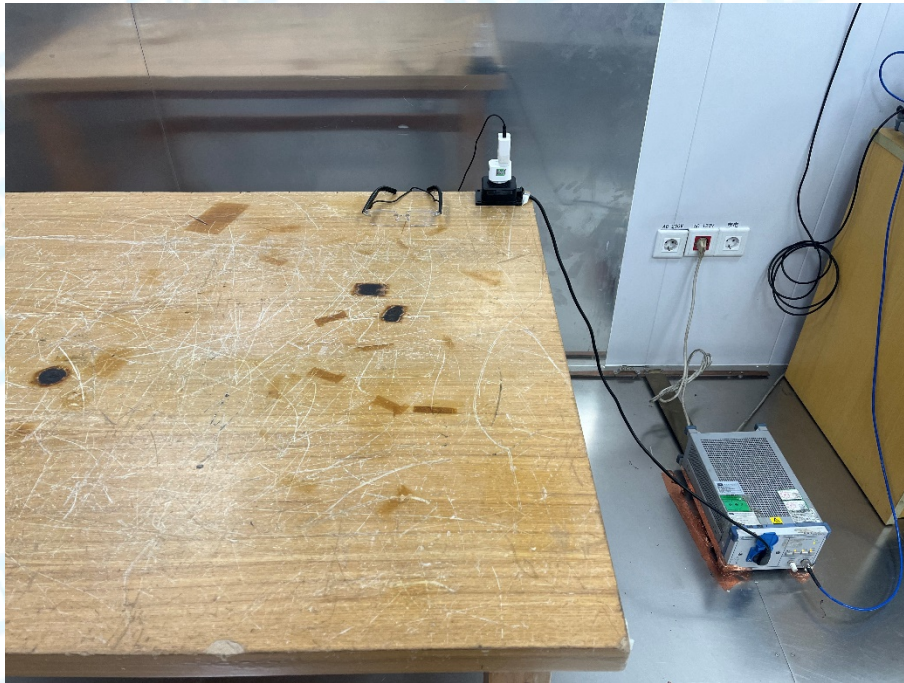
Photo of Setup for Conducted Measurement
