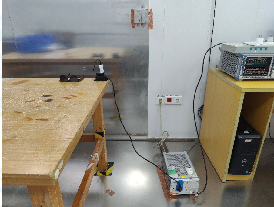
Photo of Setup for Conducted Measurement ----Left
