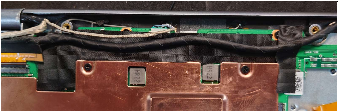
Isolate the WIFI module and the component pads on the PCB with insulating cloth.
