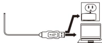
3. Insert the USB charging cable's standard USB plug into the USB port of a computer or suitable USB charging adapter.
