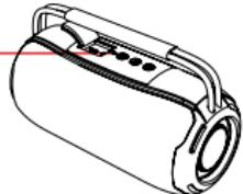
4. The LED Indicator will turn red while the speaker are charging, the red indicator light turns off after charging is completed.
