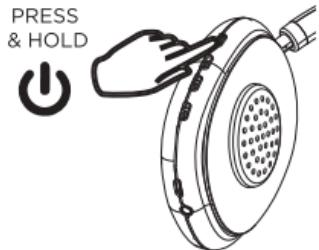
1. Press and hold the Power/Mode button for three seconds to turn the headphones On.
