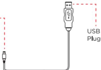
1. The USB charging cable has a Micro USB plug and a standard USB plug.
