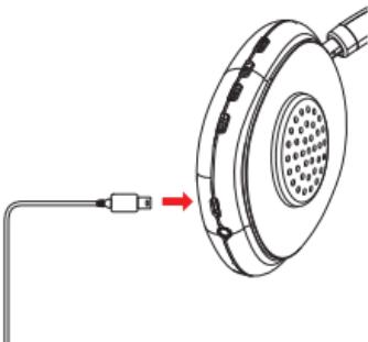
2. Insert the USB charging cable's Micro USB plug into the charging port on your headphones.
