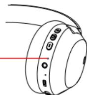
4. The LED Indicator will turn red while the headphones are charging, the red indicator light turns off after charging is completed.
