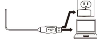
3. Insert the USB charging cable's standard USB plug into the USB port of a computer or suitable USB charging adapter.
