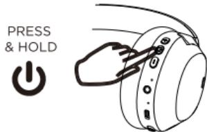
1. Press and hold the Power button for three seconds to turn the headphones On.
