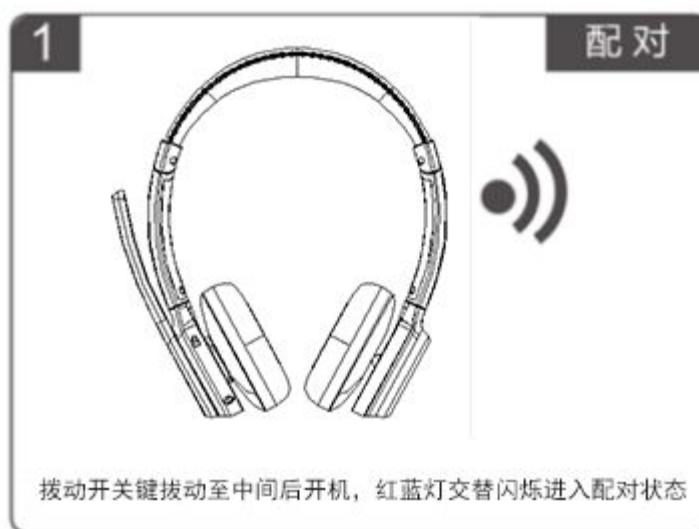
Pairing: In off state, turn the switch to the middle to enter pairing mode, with Blue & Red LED flash alternately.
