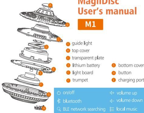
Notice: This figure shows the configuration of the host, and the function of the mate is slightly different from that of the host.
