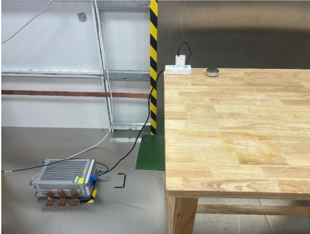
AC Power Line Conducted Emission
