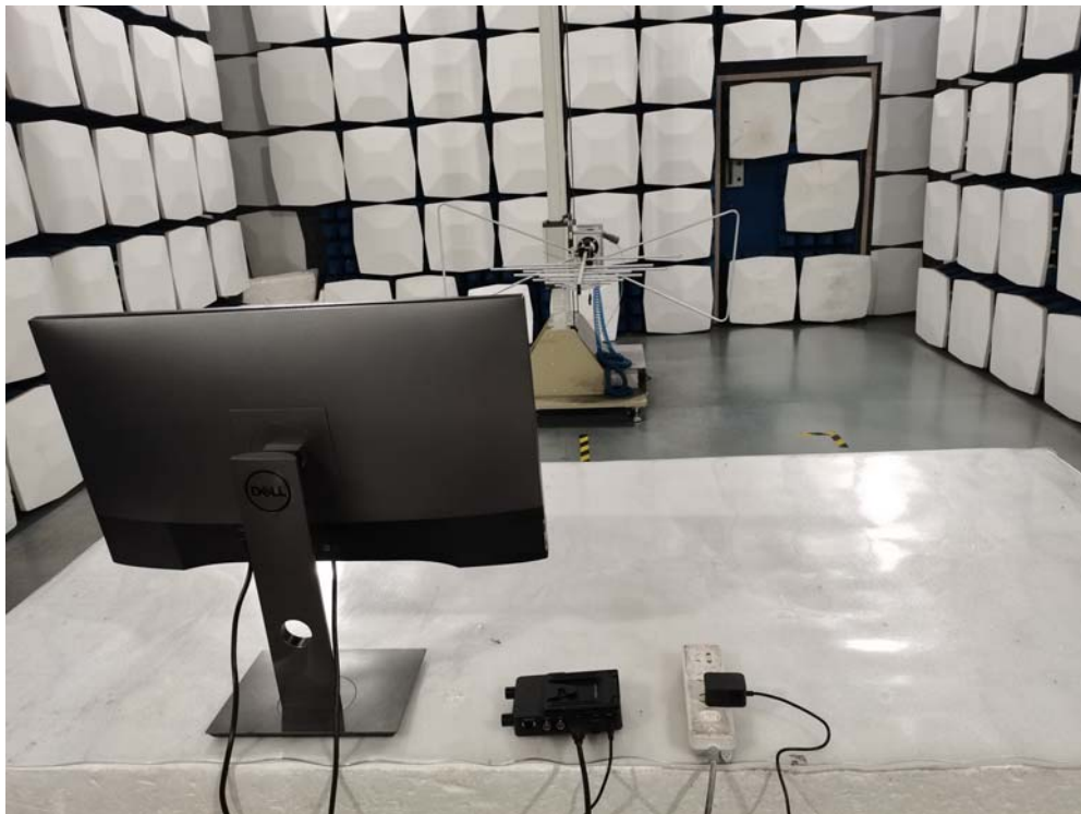
Radiated emission test view:
