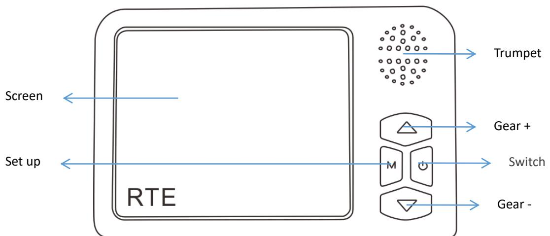
Remote control matching method: when the host is powered on, press and hold the Add key on the host and RTE will be displayed on the screen. At this time, press the+symbol key on the remote control and exit automatically after the matching is successful.
