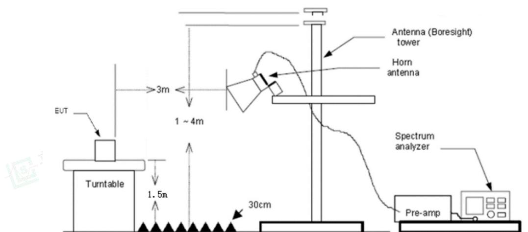
Above 18 GHz shall be extrapolated to the specified distance using an extrapolation factor of 20 dB/decade from 3m to 1m.
