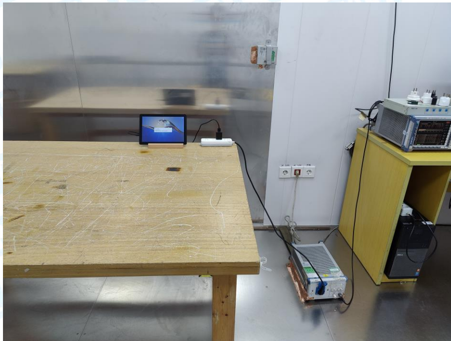
Photo of Setup for Conducted Emission
