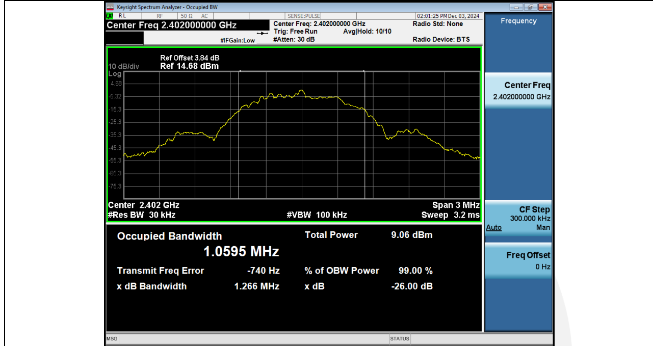
99% Occupied Bandwidth NVNT_ANT1_1Mbps_2402
