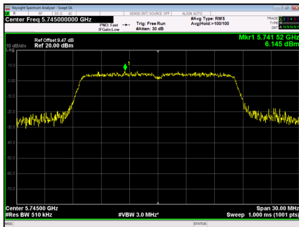
(802.11a) PSD plot on channel 157
