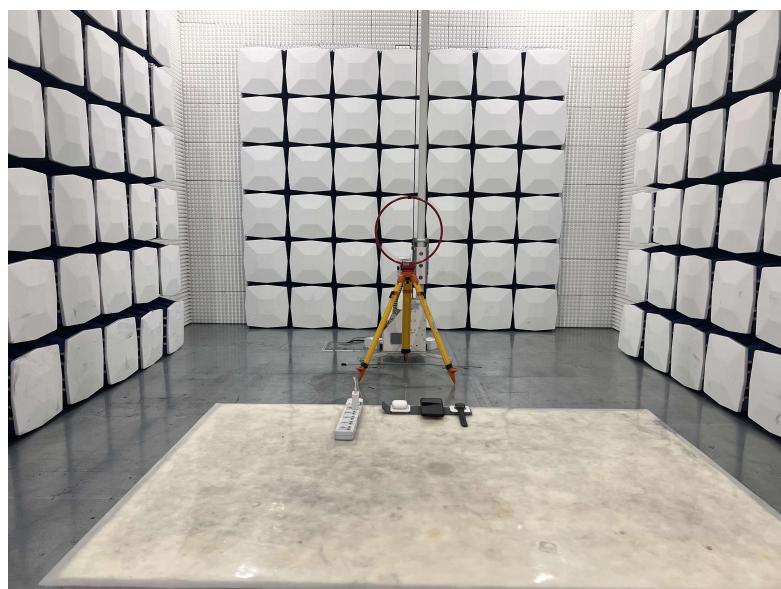
RADIATED EMISSION MEASUREMENT (below 1G)
