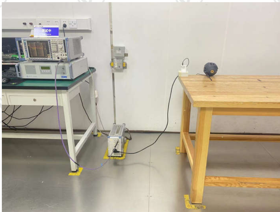
Conducted Emissions Test Setup
