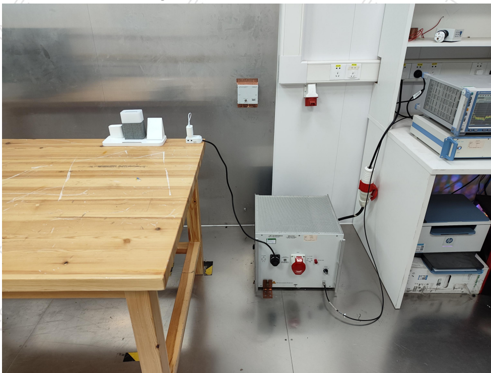
Photo of Conducted Emission Measurement
