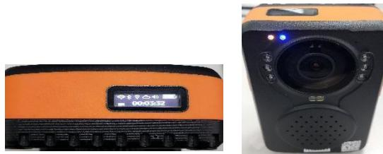
Translation: "During recording, press the recording button again to end the recording. The device will automatically save the recorded file. The screen will display the time interface, and the yellow working indicator light will turn off. The recording files are saved in the format of '20220221\_xxxx\_0001000x.mp4,' where the first 8 digits '20220221' represent the date (year, month, day), and the middle and last digits 'xxxx\_0001000x' represent the serial number. You can view or play the
