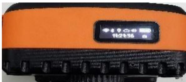
During capturing, the LCD screen will briefly display the remaining number of available photos. After capturing, it will return to the time screen, and the yellow
