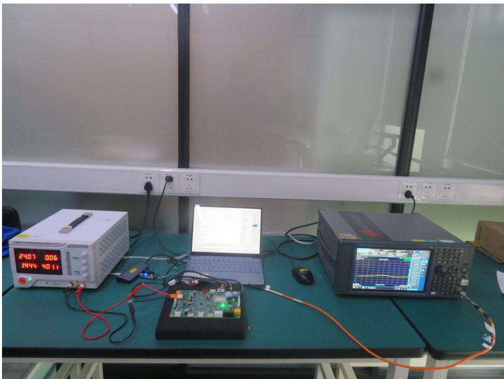
Description: Conducted Test Setup (For SRD)
