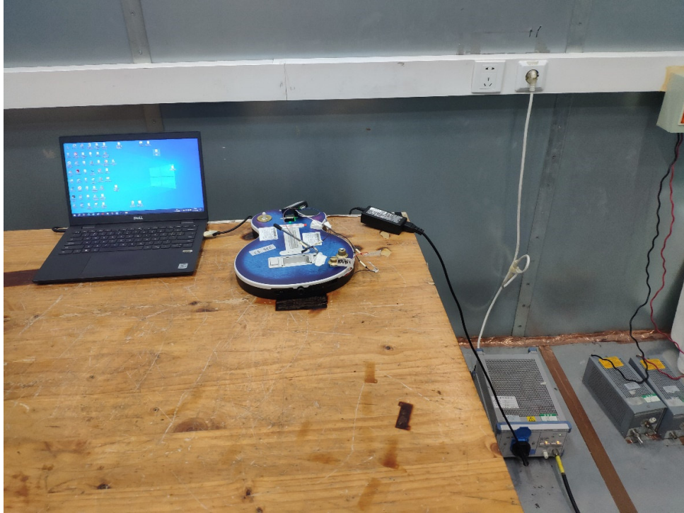
Picture 2 Conducted Emission Test Setup
