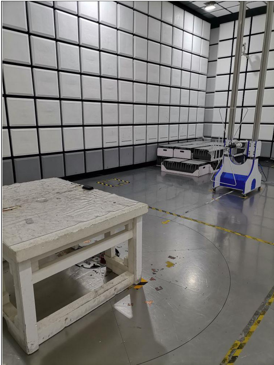
RADIATED EMISSION TEST (Below 1GHz)
