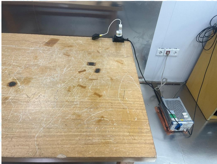
Radiated Emission Test Setup-Below 1G
