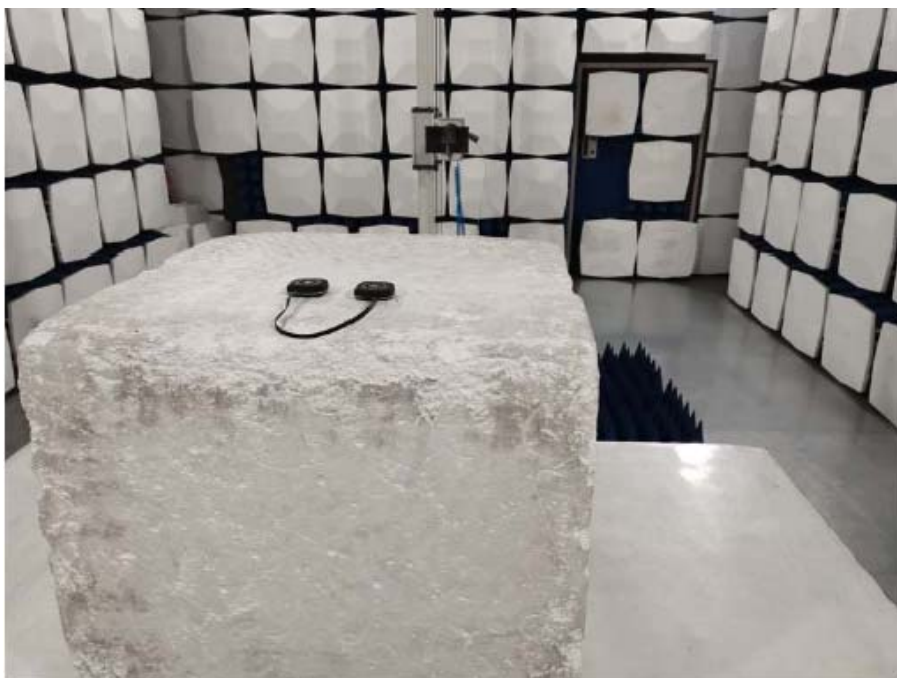
Radiated Emission Test Setup
