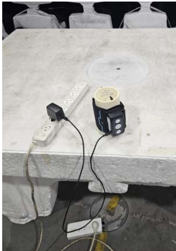
Picture # 3. EUT test setup, Charging mode
