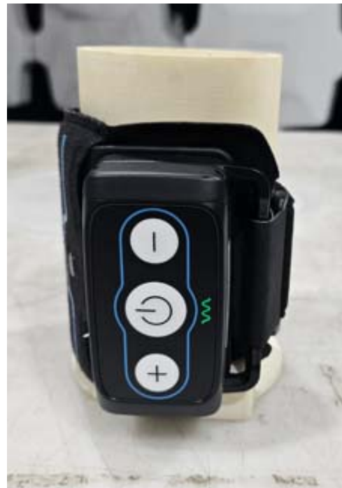
Picture # 4. Radiated emission test setup - Operation mode
