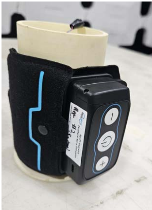
Picture # 4. Radiated emission test setup - Operation mode
