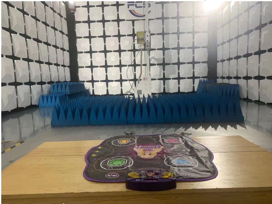
Above 1GHz for radiated emission test setup
