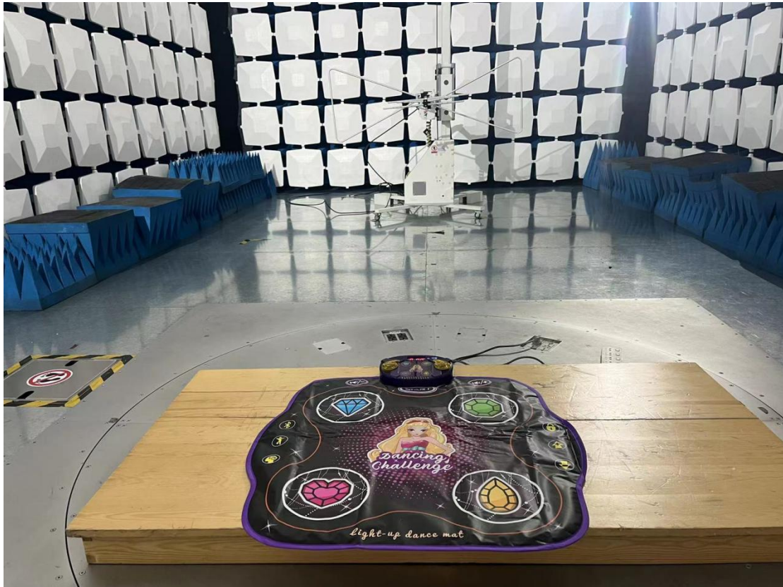
Above 1GHz for radiated emission test setup
