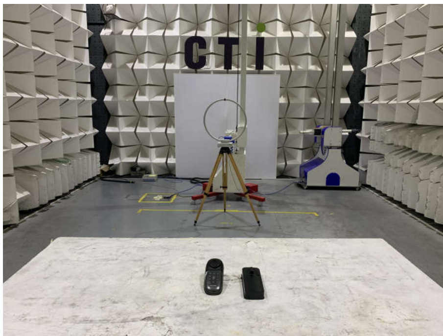
Radiated Spurious Emissions Test Setup (9kHz~30MHz)
