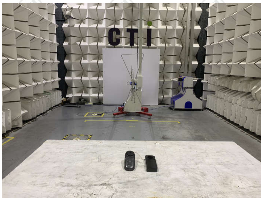
Radiated Spurious Emissions Test Setup (30MHz~1GHz)
