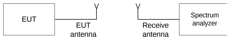
Figure 7.1.1 6 dB bandwidth test setup
