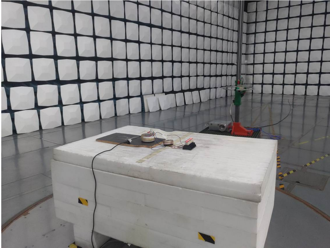
Radiated Emission 30M-1GHz View
