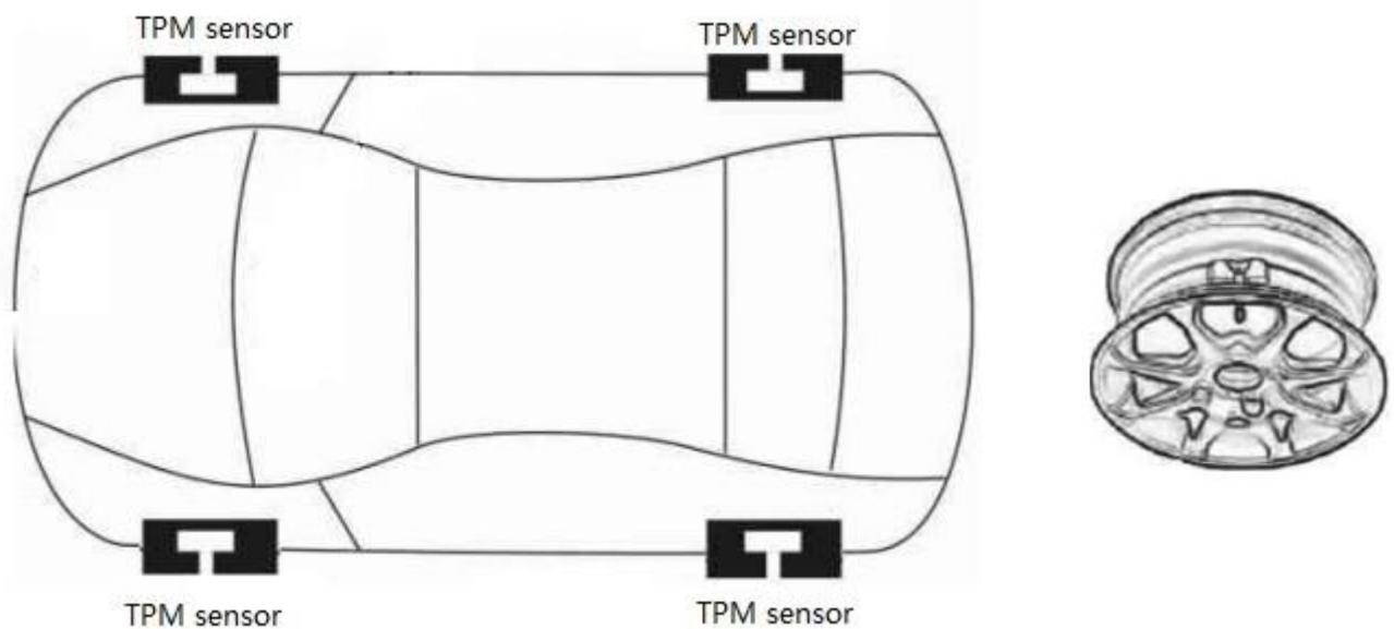
1. The sensor will be in sleep mode to save battery life. After mounter onto rim, and inflate the tyre to recommend pressure data(RCP from Car manufacturer), sensor will exit sleep mode and enter into stationary mode.
