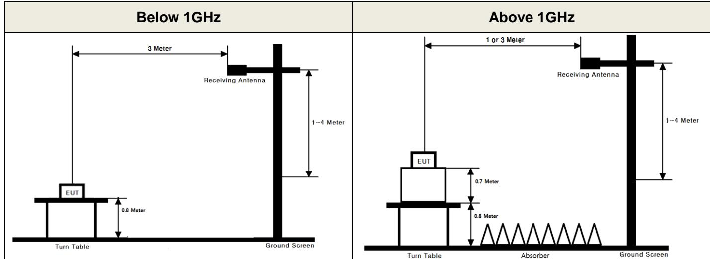
These measurements were performed at 3 m test site. The equipment under test is placed on a non-conductive table 0.8 or 1.5-meters above a turntable which is flush with the ground plane and 3 meters from the receive antenna. For measurements above 1GHz absorbers are placed on the floor between the turn table and the antenna mast in such a way so as to maximize the reduction of reflections. For measurements below 1 GHz, the absorbers are removed.
