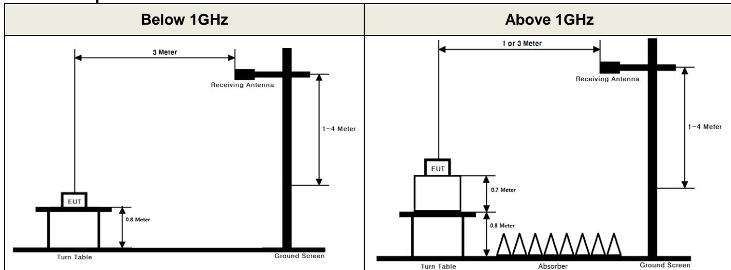
These measurements were performed at 3 test site. The equipment under test is placed on a non-conductive table 0.8 or 1.5 meters above a turntable which is flush with the ground plane and 3 meters from the receive antenna. For measurements above 1 GHz absorbers are placed on the floor between the turn table and the antenna mast in such a way so as to maximize the reduction of reflections. For measurements below 1 GHz, the absorbers are removed.
