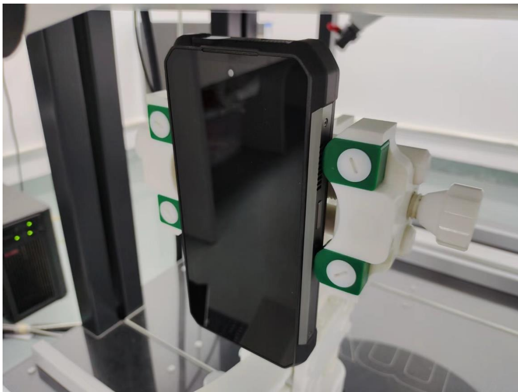
Body Top side (separation distance is 10mm)
